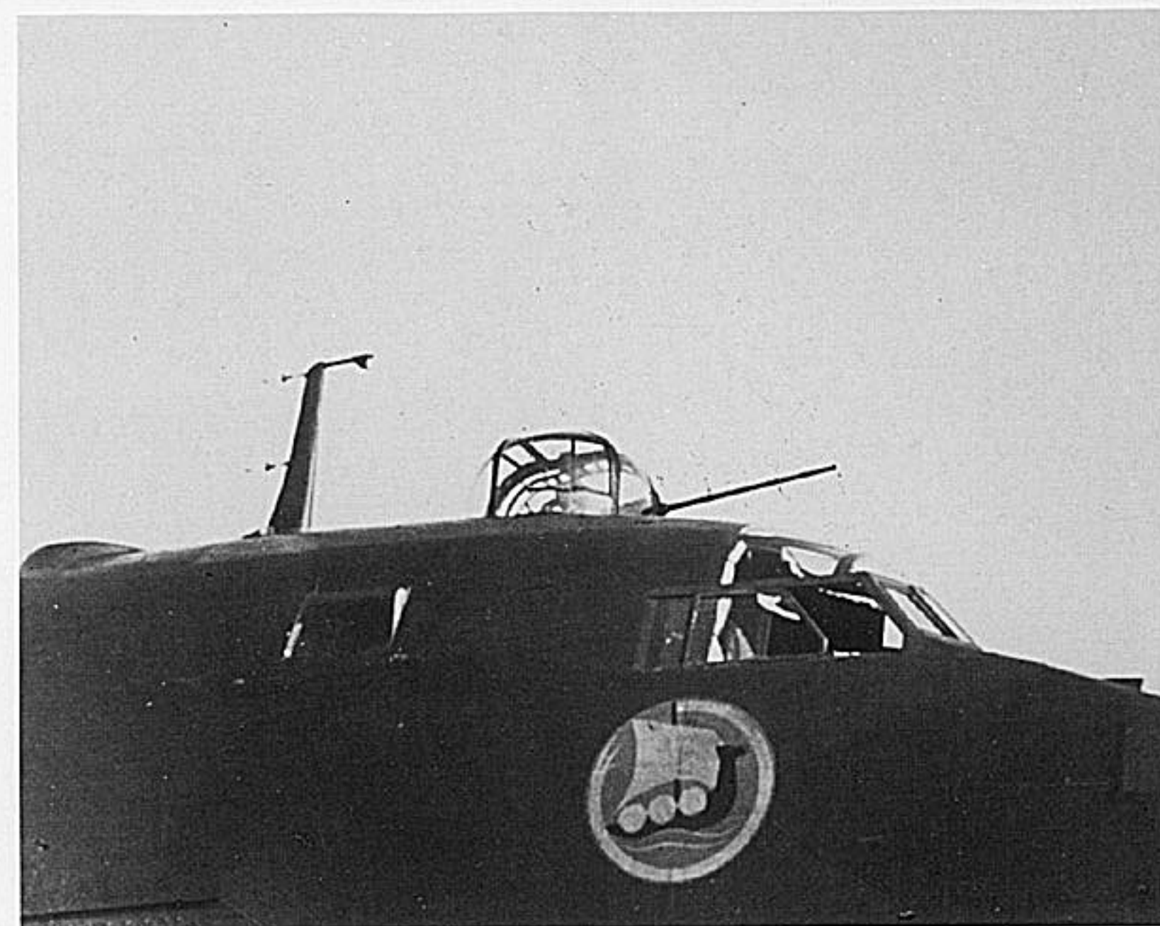
Turret and MG 151 on the upper wing of Bv 222 V 4.
